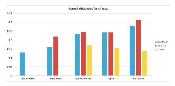
\*Note: Cold start and hot start values for Tripod are identical due to the negligible heat storage capacity of the tripod
