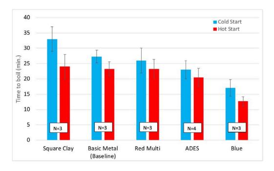
\*Note: Boiling times between stoves are not statistically different.
