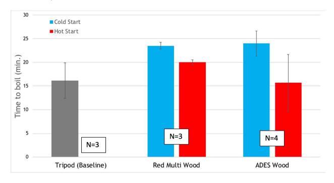
\*Note: Boiling times between stoves are not statistically different.
