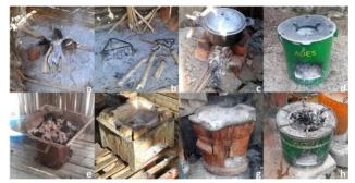
Figure 2. Examples of cooking stoves or structures, top, left to right, firewoodfueled: stone structure, metal tripod, brick structure, ADES-wood; bottom, left to right, charcoal fueled: simple metal, brick-clay stove with metal protection, brickclay stove without metal protection, ADES-charcoal.
